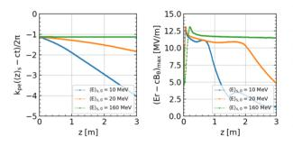
Figure 3: Initial energy dependence of seed electron bunch longitudinal centroid (left) and its wakefield amplitude (right) evaluated at  $r = 200 \,\mu m$ . Plasma starts at z =Plasma density:  $n_0 = 2 \times 10^{14} \text{ cm}^{-3}$ .
