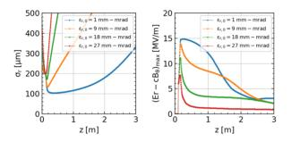
Figure 1: Evolution of the beam rms radius (left) and of the transverse wakefield amplitude evaluated at  $r = 200 \,\mu m$ (right) driven behind the seed electron beam with different initial transverse emittances. Plasma starts at z = 0.1 m. Plasma density:  $n_0 = 2 \times 10^{14} \text{ cm}^{-3}$ .
