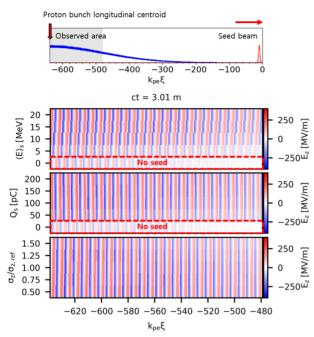
Figure 4: Phases of SSM at the longitudinal centroid of proton bunch by scanning seed beam initial energy (the second row), charge (the third row), and length (the fourth row). The seed electron beam is initially centered at  $k_{pe}\xi \approx -4.7$ . Plasma density:  $n_0 = 2 \times 10^{14} \text{ cm}^{-3}$ .
