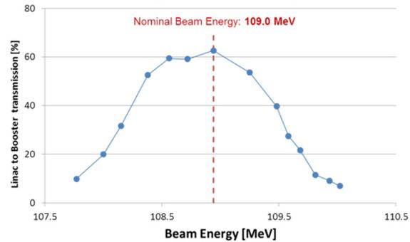
Figure 6: Booster energy acceptance window measurement. Nominal Linac beam energy centered on the window provides higher transmission stability over time.
