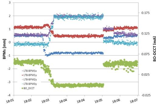
Figure 3: A forced beam misalignment at LTB reduces the beam current injected to Booster (in green). All the Beam Position Monitors (BPMs) readings are successfully brought to golden orbit when iterating over 3 corrections.
