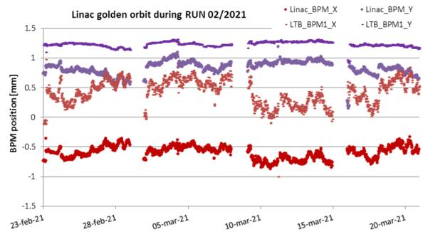
Figure 5: Linac-golden-orbit stability during RUN 2 shows a very good beam position stability. 1-to-1 orbit correction has been applied about twice per week. Orbit oscillations observed are caused by day-night temperature variations.
