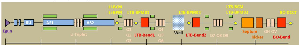
Figure 1: Schematics of the main elements involved in the optimization of the transmission at Linac, LTB and Booster. Notice the Linac cavities (blue), the quadrupoles (pink), the corrector magnets (green), the pulsed elements (orange) and the diagnostics elements (yellow).
