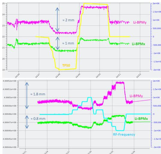
Figure 4: Beam position variations measured at Linac exit at Li-BPM. Above: when varying the 500 MHz pre-buncher phase (TPS0) by  $\pm 3^\circ$ . Below: when varying the Master Oscillator 500 MHz RF-frequency by  $\pm 2$  kHz.
