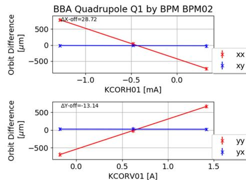
Figure 2: Horizontal (top) and vertical (bottom) magnetic center of quadrupole Q1 of the LTB. xx, xy lines in the top plot, refer to the x, y orbit variations when positioning the beam by the horizontal corrector. yx, yy lines in the bottom plot when changing the vertical corrector.
