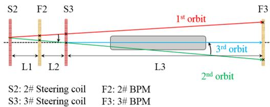
Figure 2: Correction scheme of the optical line. The black dash line in the center represents the reference optical axis.
