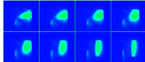
Figure 6: Beam profile on F3 when scanning the current of Q5: 1 A, 1.2 A, 1.4 A, 1.6 A, 1.8 A, 2.0 A, 2.2 A, 2.4 A.
