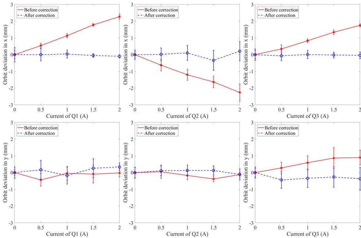
Figure 1: Beam spot drift corresponding to Q1, Q2 and Q3 before and after correction when scanning the quadrupole current.
