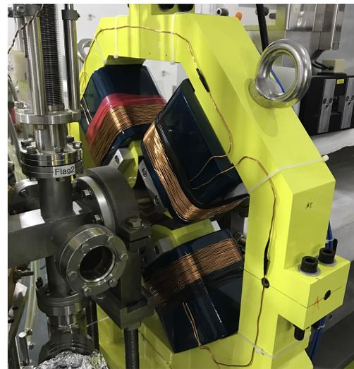
Figure 3: Vertical steering coil S3 wound on Q5.
