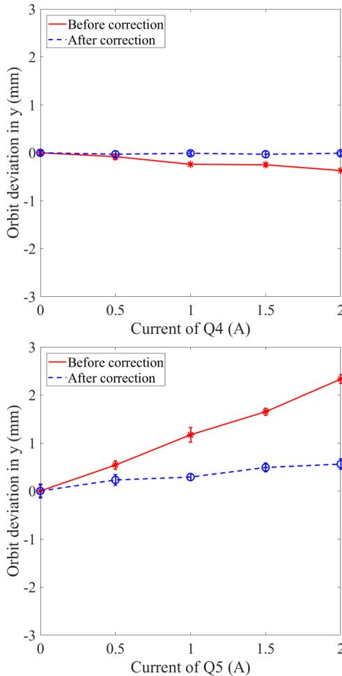
Figure 4: Vertical beam spot drift corresponding to Q4 and Q5 before and after correction when scanning the quadrupole current.
