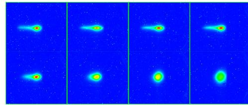
Figure 5: Beam profile on F2 when scanning the current of Q4: 0 A, 1 A, 1.5 A, 2 A, 4 A, 6 A, 8 A, 10 A.
