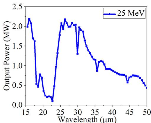
Figure 6: Simulation of FELiCHEM middle infrared laser (waveguide(a**x**b):  $30 \times 10$  mm).
