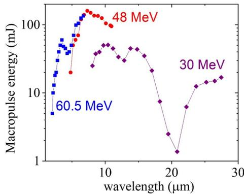
Figure 4: Macropulse energy of FELiCHEM middle infrared laser (measured by energy meter in Nov. 2020) (waveguide(a×b): 35 × 10 mm).
