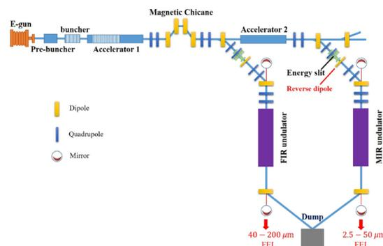
Figure 2: Schematic of FELiCHEM's FEL layout.
