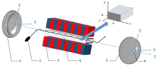
Figure 3: Schematic of FELiCHEM's MIR FELO layout.
