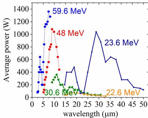
Figure 5: Average power of FELiCHEM middle infrared laser (measured by power meter in Jun. 2020) (waveguide(a×b): 20 × 10 mm).
