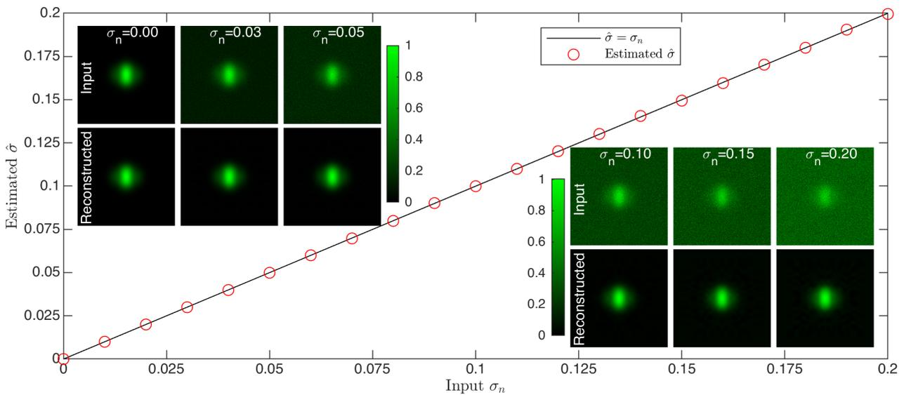
Figure 1: Mode decomposition and image reconstruction results. Gaussian noises with different levels (input  $\sigma_n$ ) are added to the same ideal beam (65% HG<sub>0,0</sub>, 20% HG<sub>0,1</sub>, and 15% HG<sub>2,0</sub>) to obtain the input images. Using these images, the modal weights and  $\hat{\sigma}^2$  are retrieved. The insets show the input and reconstructed images at different  $\sigma_n$  values.
