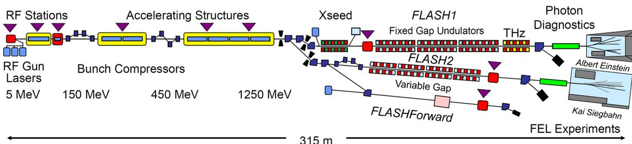
Figure 1: Schematic layout of the FLASH facility in 2021 (not to scale).
