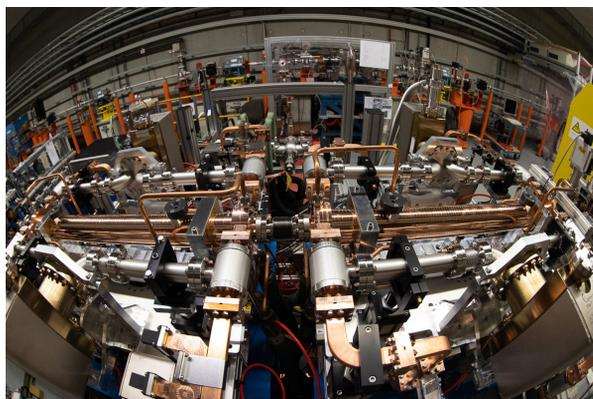
Figure 3: Top view of the two newly installed PolariX TDSs. The beam direction is from right to left, the last FLASH2 SASE undulator is visible on the right hand side (yellow girder).
