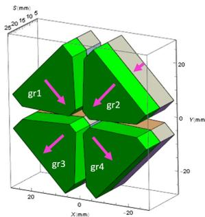
Figure 4: Half period structure of the APPLE X undulator at minimum gap with magnetization orientation for the four sub-girders.
