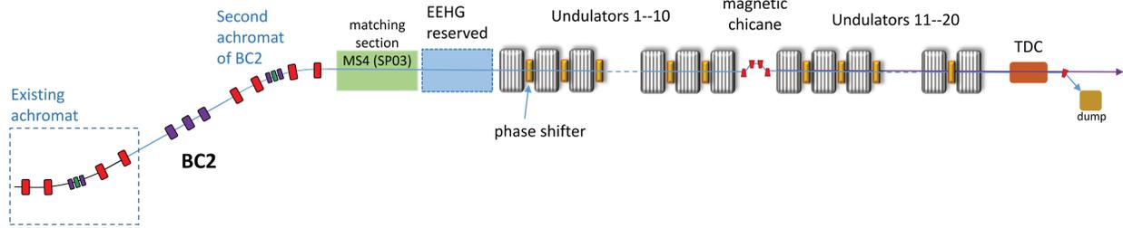
Figure 2: Layout of the SXL FEL line from the end of the last bunch compressor (BC2).
