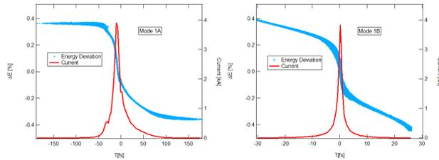
Figure 1: Longitudinal phase space. The high charge-long bunch mode (left) and low charge-short bunch mode (right).
