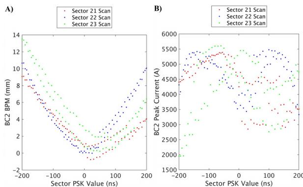
Figure 3: Plots of A) BPM in the BC2 chicane, which is proportional to electron beam energy, and B) peak current in BC2, for scanning the PSK in sectors 21, 22, and 23.
