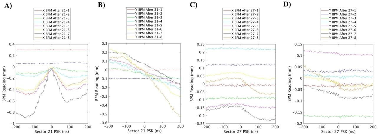
Figure 2: PSK scans for sector A-B) 21 and C-D) 27. BPM readings within the sector scanned are plotted for X and Y.
