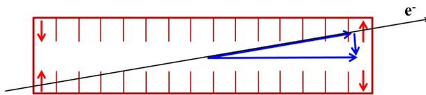
Figure 1: RF Kicks. The effects of  $R_{in}$  and  $R_{out}$  are illustrated in red, and  $R_{acc}$  is illustrated in blue.
