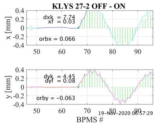
Figure 4: Difference orbit for turning on/off klystron 27-2. OrbX and OrbY give the electron orbit (in mm) in section 27-2 when the klystron is on. dXk, dYk, dXf and dYf are fit parameters (units of mm).
