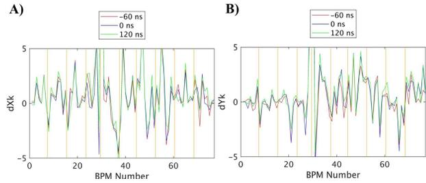
Figure 6: Fitted A)  $dX_k$  and B)  $dY_k$  for PSK = -60, 0, 120 ns. Yellow lines indicate the boundaries between accelerator sectors.
