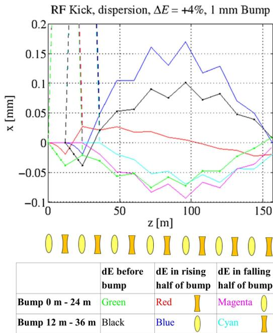
Figure 5: Simulation of a 1 mm bump in one of two locations, with an accelerating segment in one of three locations.
