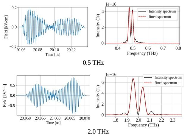
Figure 5: For the two frequencies the on-axis (LEFT) THz radiation field pulse and (RIGHT) on-axis spectral field and intensity plot.
