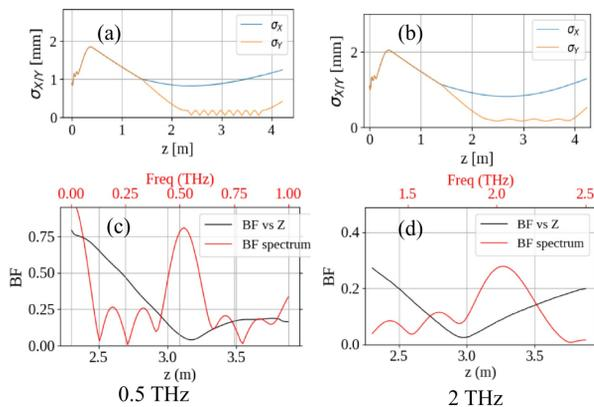
Figure 2: Simulation result for 0.5 and 2 THz showing the (a, b) transverse rms beam size variation and (c, d) the BF spectrum (in red) at undulator and the BF variation through the undulator at said frequency.
