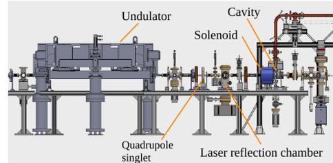
Figure 1: The beamline design of DLS upto undulator.
