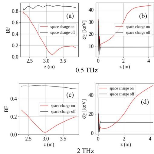
Figure 4: For the two frequencies, the variation of BF through undulator (a,c) and the energy spread variation (b,d) simulated with and without space charge.
