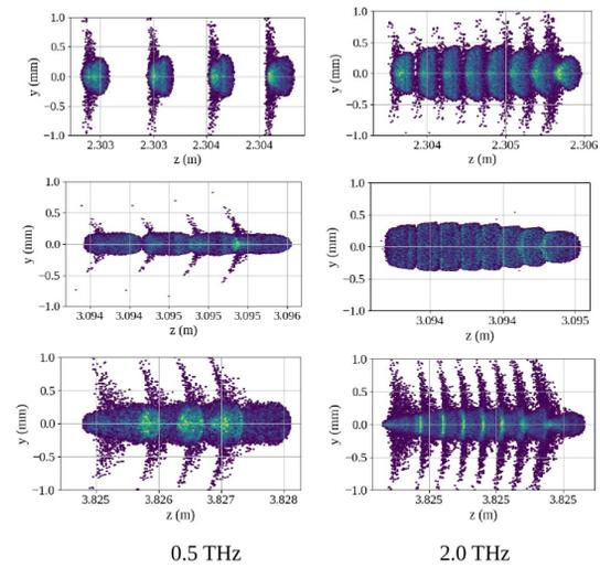
Figure 3: For the two frequencies the longitudinal profile at (TOP) undulator start, (MID) undulator middle and (BOTTOM) at undulator exit.
