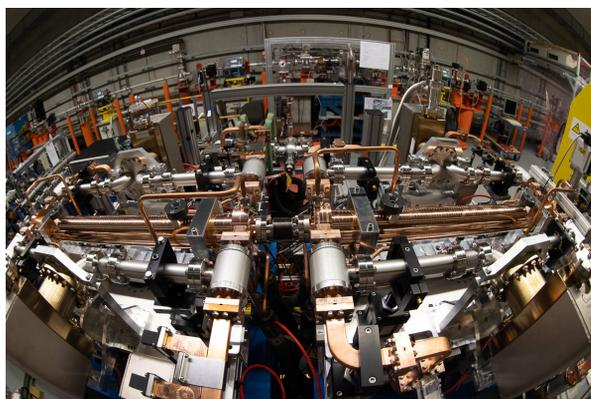
Figure 3: Top view of the two newly installed PolariX TDSs. The beam direction is from right to left, the last FLASH2 SASE undulator is visible on the right hand side (yellow girder). Image courtesy of D. Nölle.
