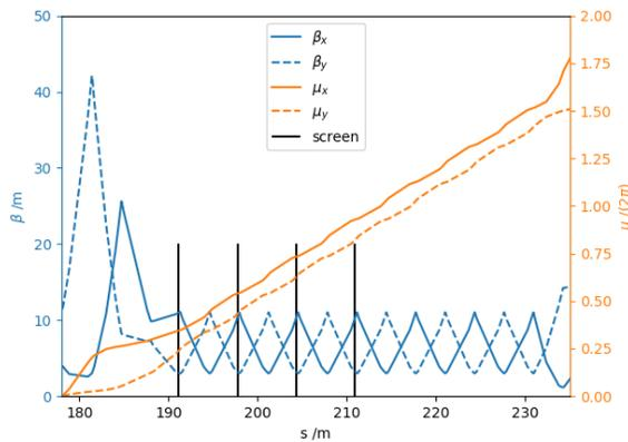
Figure 6: Optical functions proposed for matching into the FLASH2 undulators using a four screen method. The phase advance between the screens is  $\Delta\Phi_{x,y} = 70^\circ$ .
