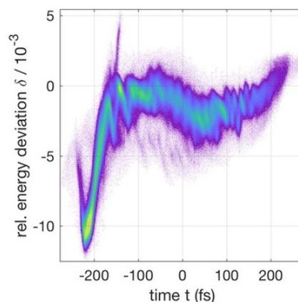
Figure 4: Example of first measurements of the LPSD with the newly installed PolariX at FLASH2. The resolution achieved with an RF input power of 3 MW was 10 fs, which is already impressive.
