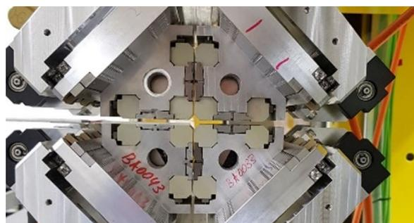
Figure 5: Picture of the APPLE III afterburner prototype. Each of the four quadrants can be moved longitudinally to change the polarization. Image courtesy of M. Tischer.
