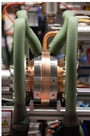
Figure 2: X-band barrel open pulse compressor (XBOC) used to quadruple the power coming from the klystron. Image courtesy of D. Nölle.
