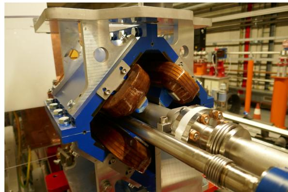
Figure 1: Quadrupole downstream of the separation of the photon and the electron beamline. The photon beamline is inside of the iron yoke of the magnet.
