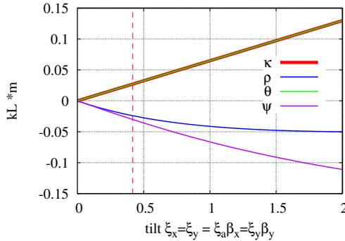
Figure 3: Correcting integrated quadrupole strengths  $\kappa$ ,  $\rho$ ,  $\theta$ , and  $\psi$  for the case with all  $\xi_i \neq 0$  and typical FLASH2020+ parameters. The vertical red broken line is the expected tilt for FLASH2020+.
