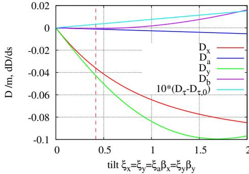
Figure 4: Leaking dispersions  $D_x$ ,  $D_a$ ,  $D_y$ ,  $D_b$ , and the change of momentum compaction  $D_\tau - D_{\tau,0}$  at the chicane exit for the case with all  $\xi_i \neq 0$  and typical FLASH2020+ parameters. The vertical red broken line is the expected tilt for FLASH2020+.
