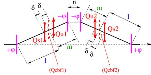
Figure 2: Layout of thin lens BCC model.
