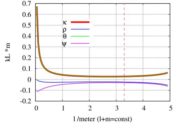
Figure 5: The dependence of the correcting quadrupole strengths  $\kappa$ ,  $\rho$ ,  $\theta$ , and  $\psi$  on the location of the quadrupole pack inside the chicane leg (vary  $l$  with  $l + m = \text{const.}$ ). The vertical red broken line is the  $l$  of the FLASH2020+ design.
