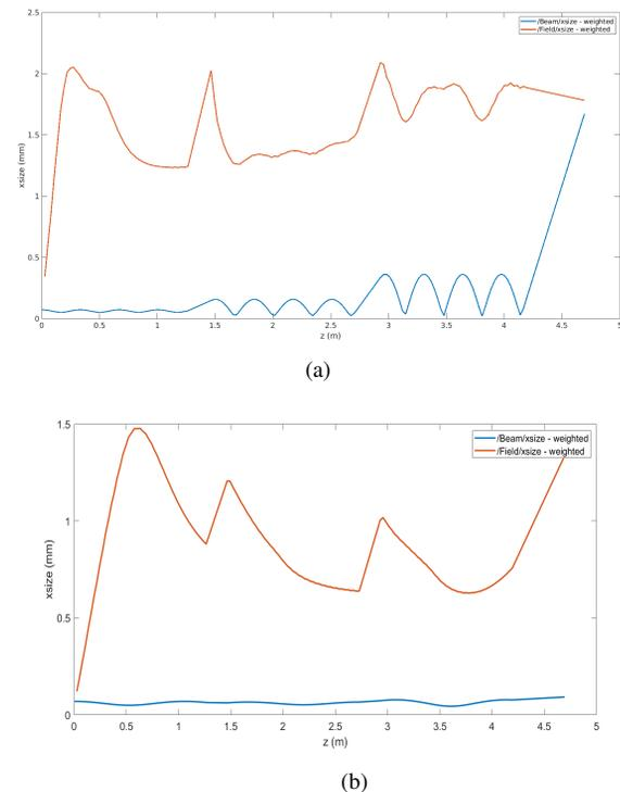
Figure 1: Genesis 1.3 simulations of beam (blue) and radiation (red) rms size along the undulator along x direction (the y direction is analogous because of APPLE-X symmetric focusing properties): (a) 100  $\mu\text{m}$  radiation wavelength case; (b) 10  $\mu\text{m}$  radiation wavelength case.
