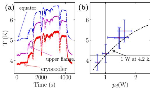
Figure 5: Thermometers reading at 3 different locations during the test (a), and performance curve of the cryocooler (b).
