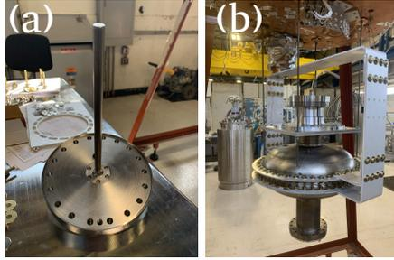
Figure 2: Photo of the Nb rod and the flange (a) and cavity and thermal links (b) during assembly.
