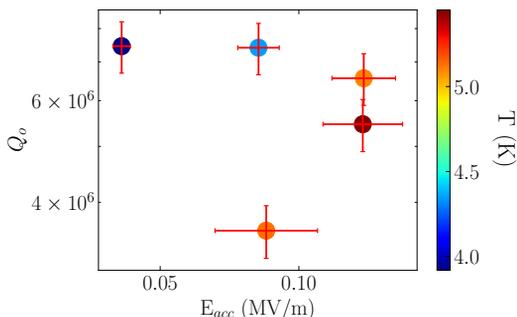
Figure 4: Average accelerating gradient  $E_{acc}$  versus the quality factor of the cavity-rod assembly  $Q_o$ . The color represent the operating temperature of the cryocooler.
