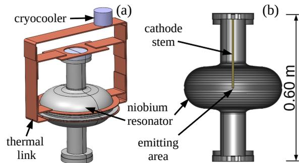
Figure 1: A 3D rendition of the modified single-cell 650-MHz cavity (a) and associated sectional view (b).
