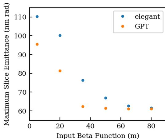
Figure 2: The dependence of the final slice emittance on the input Twiss beta function is shown as obtained from elegant and from GPT.
