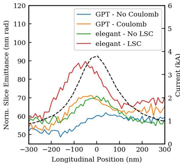
Figure 3: The slice emittance as predicted from GPT and elegant with and without their respective inclusion of Coulomb effects is plotted for  $\beta = 10$  m. The black dashed line shows the current profile.
