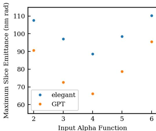
Figure 1: The dependence of the final slice emittance on the input Twiss alpha function is shown as obtained from elegant and from GPT.
