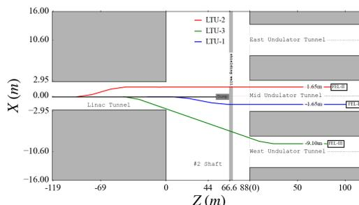
Figure 1: Layout of the beam distribution section of SHINE.
