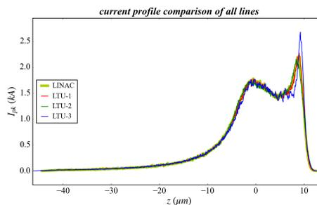
Figure 8: Comparison of the current profile at the exit of each LTU branch.
