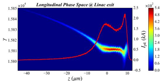
Figure 6: Longitudinal phase space at the exit of linac.
