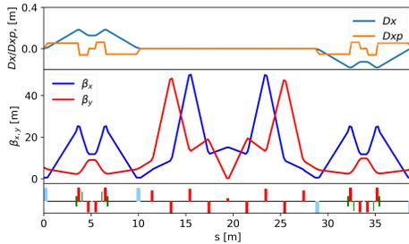
Figure 3:  $\beta$  functions and dispersion functions of the dog-leg.
