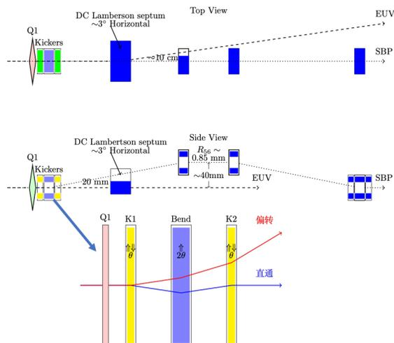
Figure 9: Resonant kicker set and DC Lamberson septum scheme for two bunch mode operation.
