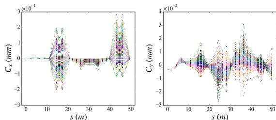
Figure 7: Transverse position jitter of 100 cases of magnet power supply jitter.
