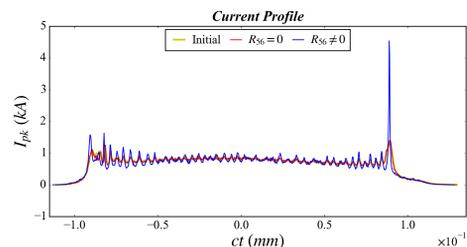
Figure 6: Comparison of the current profile before and after passing through the beam switchyard.
