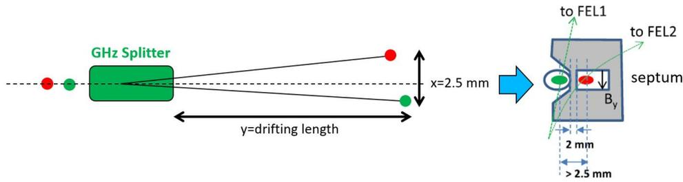
Figure 1: Schematic figure of the S-band splitter system.
