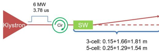
Figure 6: Schematic figure of the standing-wave deflector system with circulator. The length of the 3-cell standing-wave structure is 0.15 m and the drifting length is 1.66 m. The length of the 5-cell standing-wave structure is 0.25 m and the drifting length is 1.29 m.
