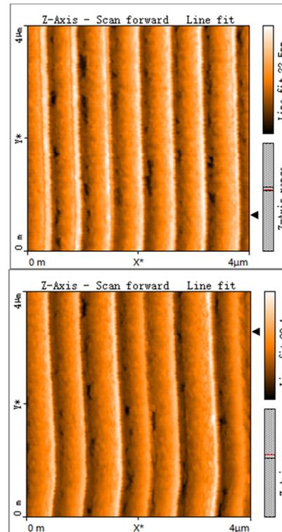
Figure 4: The measurement results of cylindrical VLS blazed grating.
