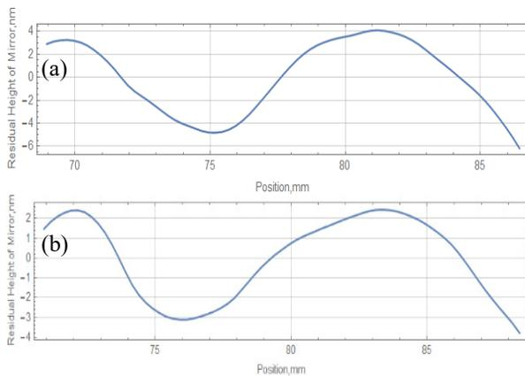
Figure 5: The measurement results of taking 17.5 mm as the optical clear length for two coatings: (a): B<sub>4</sub>C, (b): Au.
