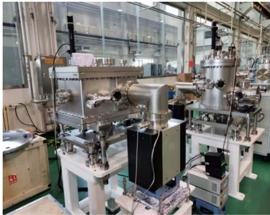
Figure 2: The outside view of the vacuum cavities of soft X-ray self-seeding.
