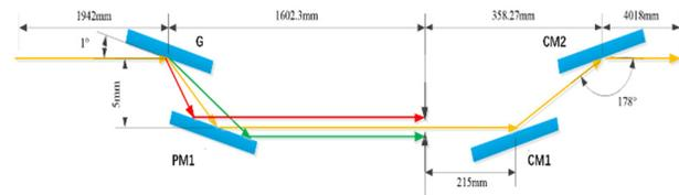
Figure 1: The layout of soft X-ray self-seeding monochromator.
