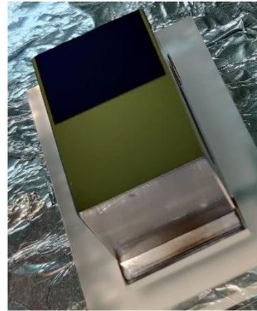
Figure 3: The picture of real VLS grating with two coating materials.
