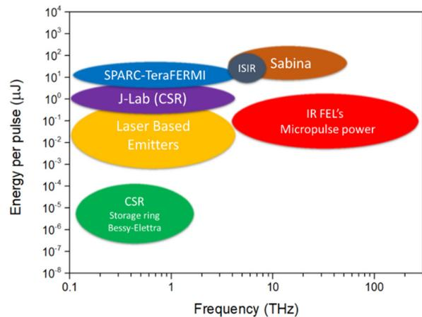
Figure 2: Energy per pulse THz/IR emission for different high-intensity ps long sources.
