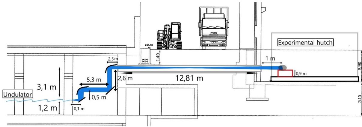
Figure 1: Beamline setup (not on scale). Light propagation is represented from the undulator source to the laboratory. M1 is plane OTR screen, M2 is an off axis parabolic mirror that collimates the beam to a plane mirror (M3). The radiation is focused by M4 into a long conduct where in the center is placed the diagnostic setup. M5, a parabolic mirror identical to M4, collimates the beam directing it to the experimental room.
