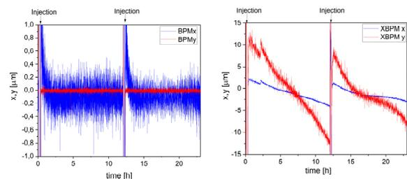
Figure 1: The BPM and XBPM readings over a time during two runs.
