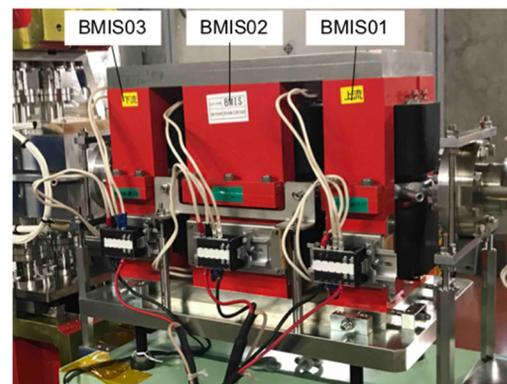
Figure 3: Chicane magnet installed in the cERL.
