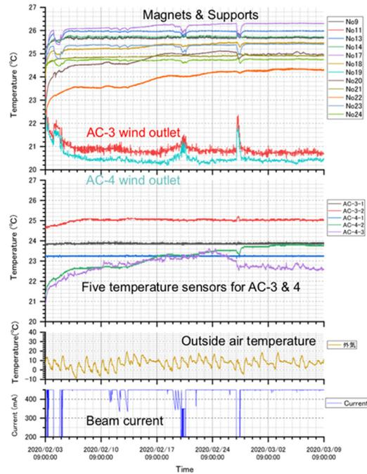
Figure 9: Temperature measurements from February to March 2020 with twelve Pt thermometers.
