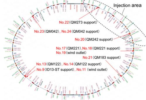
Figure 7: Twelve Pt thermometers for temperature measurement of three magnets and seven supports and AC-3 and AC-4 wind outlets.
