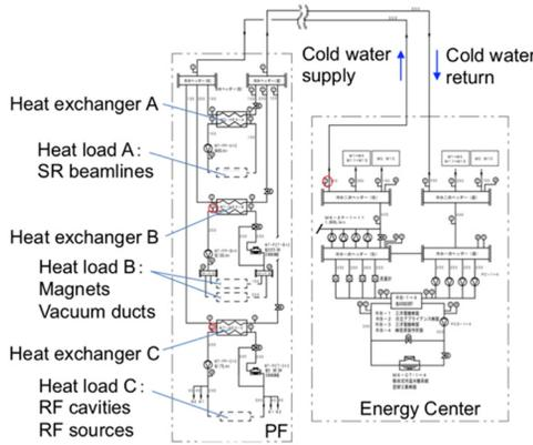
Figure 4: Schematic view of the cooling-water systems for the PF ring.
