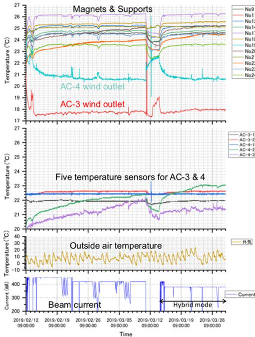
Figure 8: Temperature measurements from February to March 2019 with twelve Pt thermometers.
