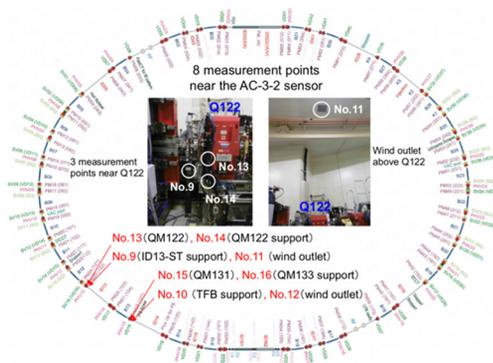
Figure 5: Eight Pt thermometers in the ring tunnel for temperature measurement of two magnets, four supports and two AC-3 wind outlets near the AC-3-2 sensor.
