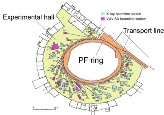
Figure 1: Layout of the PF Light Source Building. The orange area shows the tunnel of the PF ring including a part of the beam transport line from the injector linac and the yellow area the experimental hall with SR beamlines.
