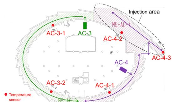
Figure 3: Layout of two air-conditioning systems (AC-3 and AC-4) for the PF-ring tunnel and the airflow directions in the air ducts. Five temperature sensors (two for AC-3 and three for AC-4). One sensor for each air-conditioner is used for the temperature FB control.
