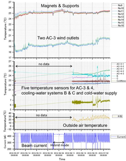
Figure 6: Temperature measurements from May to July 2018 with eight Pt thermometers.
