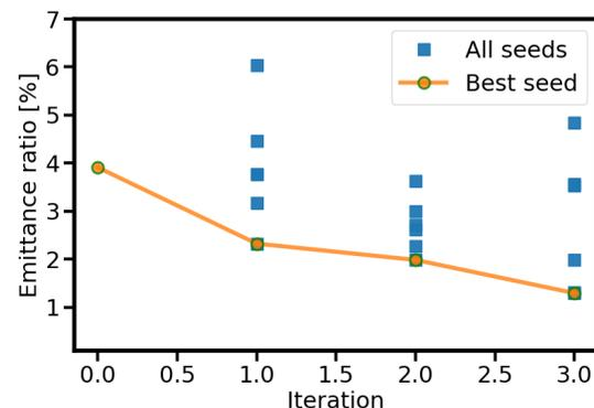
Figure 1: Online optimization of transverse emittance ratio by tuning skew quadrupole magnets current. There are 3 iterations with 6 seeds per iteration, showing best seed and all seeds.
