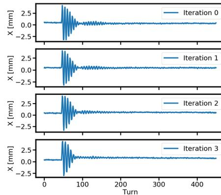
Figure 9: Turn-by-turn BPM at each iteration, showing the “best” with minimum penalty.
