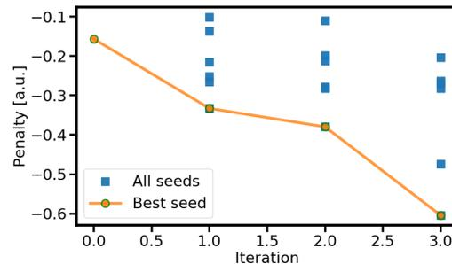
Figure 4: Optimizations on injection efficiency of a single bunch, by tuning 28 families of sextupole magnets in sectors hosting the minimum physical aperture and the four injection kickers.
