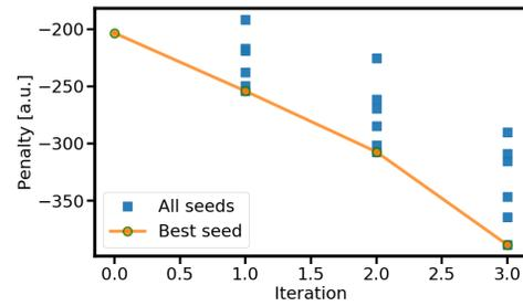
Figure 8: Online optimization of horizontal oscillation amplitudes from turn-by-turn BPMs by tuning sextupole magnets current.
