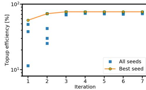
Figure 3: Optimizations of topup injection efficiency, by tuning septum and kickers voltage, plus kickers timing.
