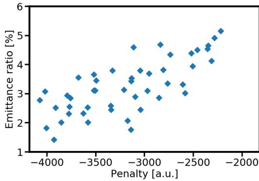
Figure 2: Transverse emittance ratio of all the seeds, versus sum of beam loss, with optimization objective of sum of beam loss.
