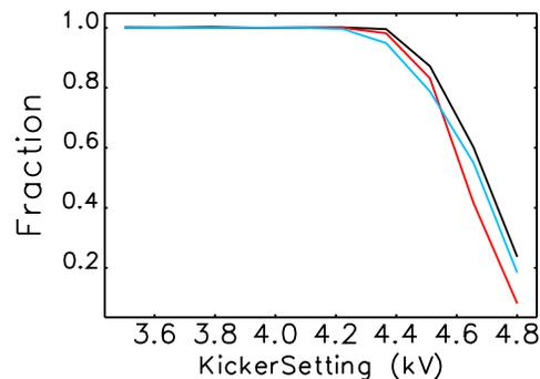
Figure 5: Measured kick apertures of nominal operation lattice (red curve), and the optimized solutions (black and blue curves) with improved injection efficiency.
