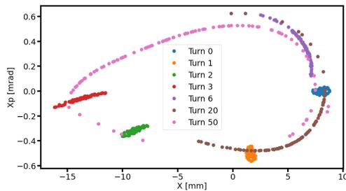
Figure 6: Horizontal phase space from 6D tracking, bunch shown for different number of turns.
