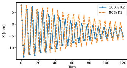
Figure 7: Bunched beam (100 macro particles) simulation illustrates decoherence effect due to tune shift with transverse amplitude.
