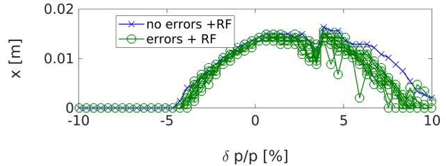
Figure 7: Off-energy max( $x>0$ ) dynamic aperture for 10 lattices with errors of 70  $\mu\text{m}$  rms in all magnets and corrections.
