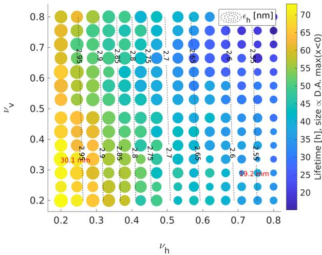
Figure 6: Average momentum acceptance and D.A. at injection vs tune working point. The size of the circles is proportional to the horizontal negative DA; the maximum and minimum are marked by red text.
