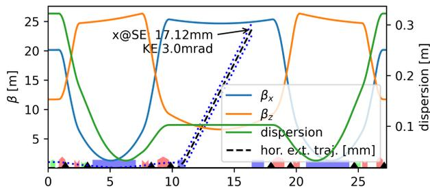
Figure 3: Trajectory of extracted beam in the horizontal plane. A 3 mrad kick displaces the beam at the septum by more than 17 mm.  $3\sigma$  envelope is also displayed with blue dashed lines.
