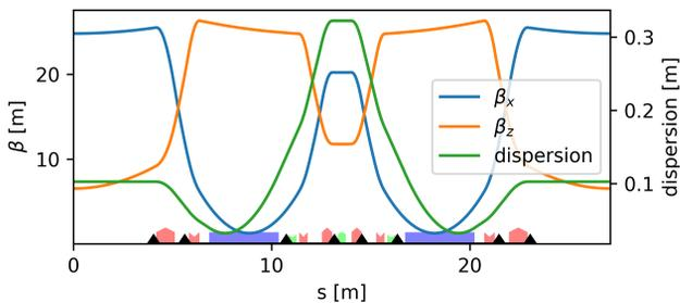
Figure 1: Magnets layout for a 40 cells DBA booster injector. Only 2 sextupole families will be required.
