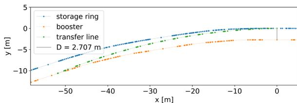
Figure 2: Survey of the extraction-injection region of the USSR facility considering a full energy booster in the same tunnel as the main storage ring.
