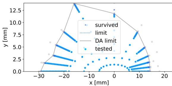
Figure 4: On-energy dynamic aperture starting at center of straight section and tracking a 6 GeV beam for 1024 turns.
