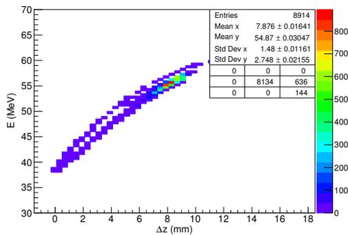
Figure 6: The longitudinal phase space of the electron bunch at the end of the accelerating cavity
