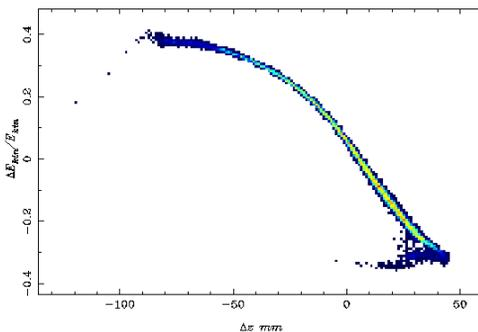
Figure 3: The longitudinal phase space of the electron bunch at the end of the SHB2.
