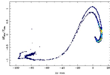
Figure 5: The longitudinal phase space of the electron bunch at the end of the main-buncher.
