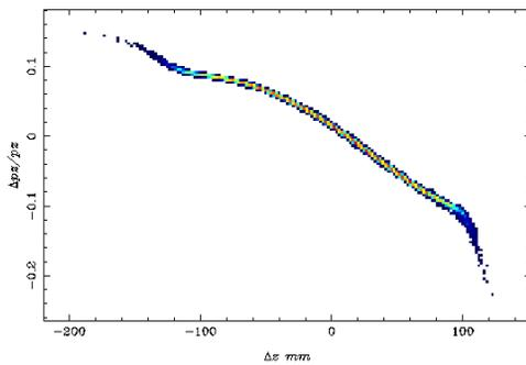
Figure 2: The longitudinal phase space of the electron bunch at the end of the SHB1.
