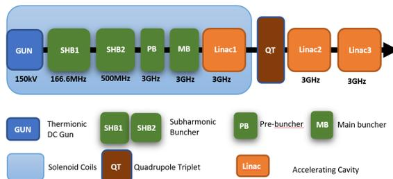
Figure 1: The layout of the low energy linac system.
