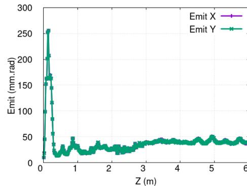
Figure 8: The transverse emittance along the bunching section.
