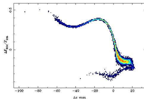
Figure 4: The longitudinal phase space of the electron bunch at the end of the pre-buncher.
