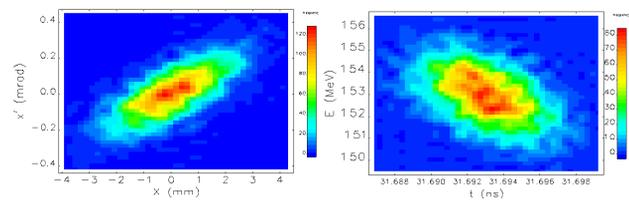
Figure 9: The transverse and longitudinal phase space at the end of the accelerating section.
