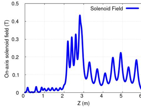
Figure 7: The on-axis solenoid field along the bunching section.
