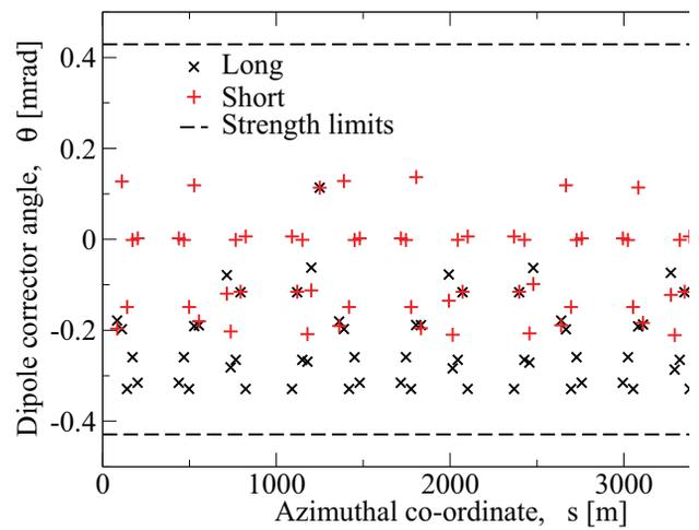
Figure 3: Dipole corrector angles used in the 2021 RHIC beam studies, with  $\delta_B = -0.01$  and before correction of random closed orbit errors. The long and short configurations have angles of  $\theta = -0.228 \pm 0.096$  mrad and  $-0.062 \pm 0.102$  mrad, respectively, well within the angular strength limits at 275 GeV indicated by the dashed lines.
