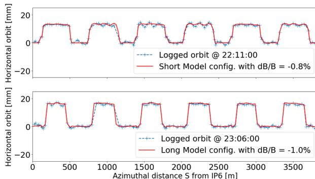
Figure 4: Closed orbits (on-axis in the IRs) measured in 2021 with 7.3 GeV/u gold beam. Top: short configuration with  $\delta_B = -0.008$ . Bottom: long configuration with  $\delta_B = -0.010$ . Model and observation are in excellent agreement when the RF frequency  $f$  is well-matched. Arc displacements as large as +23 mm have been achieved.
