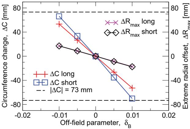
Figure 2: Configurations with shorter on-axis regions are more efficient at generating  $\Delta C$ , so larger  $|\delta_B|$  values are necessary when the on axis regions are longer. Closed orbits have the same  $\Delta R_{\max}$  values for a given  $\delta_B$ , independent of the on-axis region length. Dashed lines show the most challenging  $\Delta C$  requirements, at 100 and 275 GeV.
