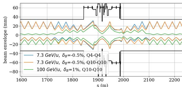
Figure 1: RHIC gold beam study envelopes. Orange and blue ( $5\sigma$  plus separatrix) indicate the “long” and “short” configurations tested in 2021 with  $\Delta B/B = \pm 0.005$ . The green envelope ( $10\sigma$  plus separatrix) is planned for future studies with 100 GeV/u gold beam and  $\Delta B/B = \pm 0.01$ .
