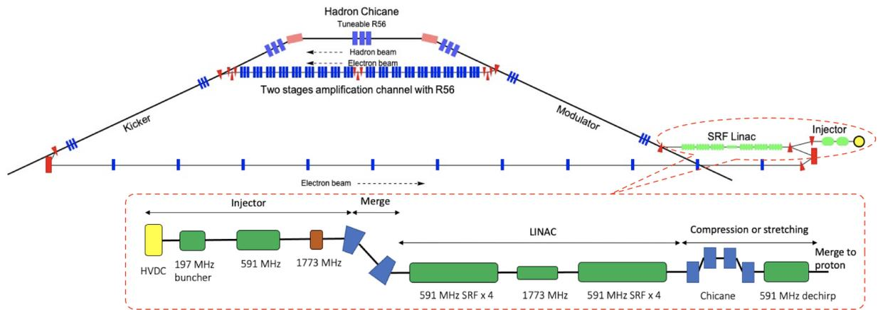
Figure 1: A schematic of strong hadron cooling accelerator and a schematic drawing of the gun to electron-proton merger.
