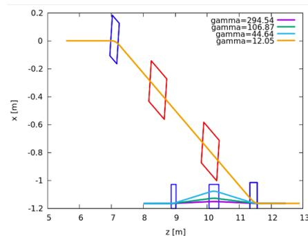
Figure 2: The lattice of the Dogleg merger with dual solenoid. It also shows three energies' trajectories merging into the LINAC.
