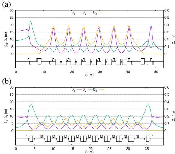
Figure 1: Optical functions of (a) 1/6 3h3l lattice and (b) 1/8 10BA lattice.
