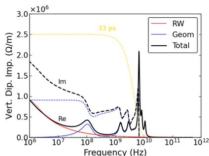
Figure 4: Vertical impedance as a function of frequency.
