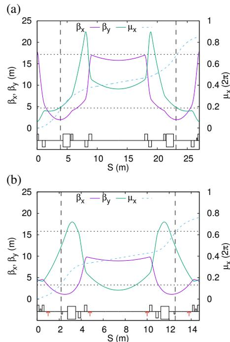
Figure 2: Optical functions in (a) high beta straight in 3h3l lattice and (b) straight in 10BA lattice.
