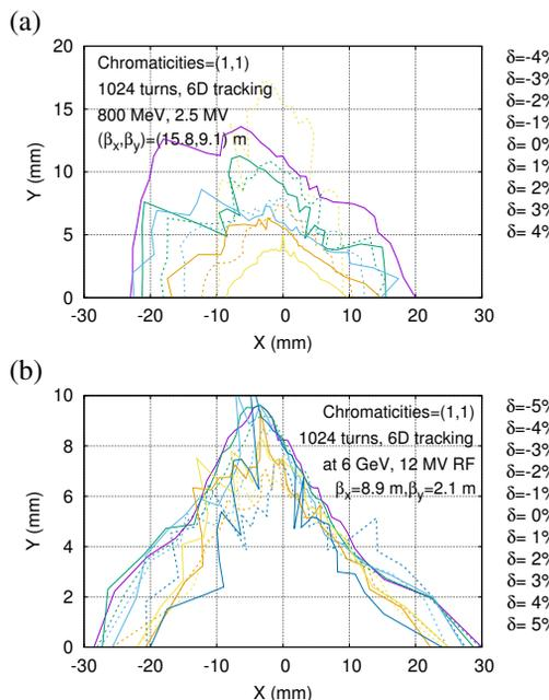
Figure 3: Dynamic apertures (a) 3h3l and (b) 10BA lattice.
