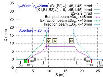
Figure 6: Orbits at injection/extraction straight.
