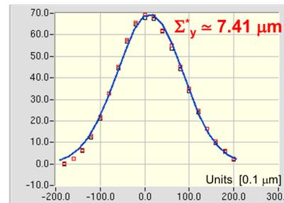
Figure 6: Vertical beam-beam luminosity scan.
