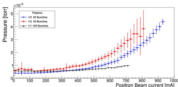
Figure 2: Positron ring vacuum rise as a function of the stored current for different bunch patterns. Each series represent the average (markers) and RMS (bars) over several hours of running.
