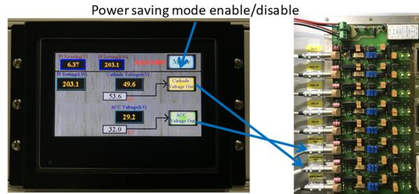
Figure 5: The man-machine interface touch panel can display the read klystron RF forward power and the output analogue signals which control the operation high voltages of klystron.
