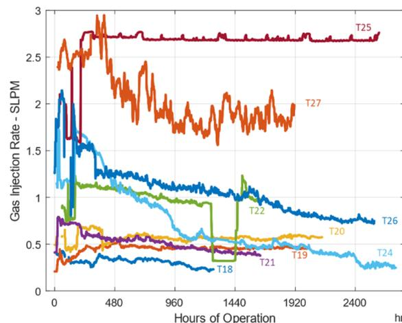
Figure 3: Gas injection flow rates for SNS targets.
