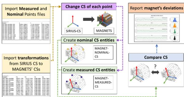
Figure 3: Workflow for data treatment and preparation.
