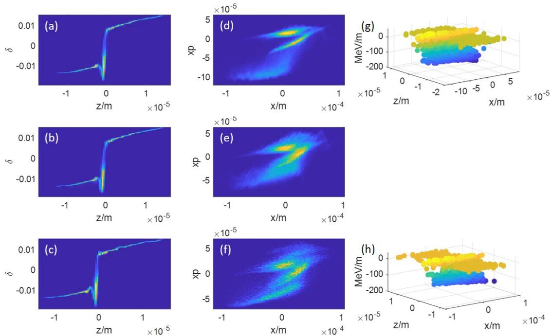
Figure 3: Longitudinal(a-c), transverse phase space(d-f) and longitudinal CSR wake(g,h) of the beam at the end of the last dipole of FACET-II upgraded BC20 chicane.(a), (d), (g) are results from our 2D model, (b), (e) from our 2D model with CSRtrack transverse wake, (c), (f), (h) from CSRtrack.
