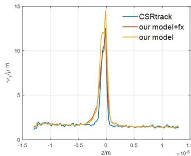
Figure 2: Slice emittance at the end of the last dipole of FACET-II upgraded BC20 compressor from CSRtrack(blue), our 2D model(yellow) and our 2D model with transverse force from CSRtrack(red).
