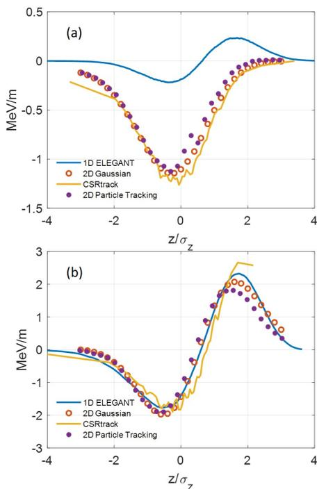
Figure 1: Longitudinal CSR wake along the central axis of the beam in the middle of the third (a) and fourth (b) bend of the benchmark chicane.
