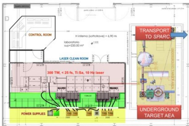
Figure 3: FLAME schematic layout.
