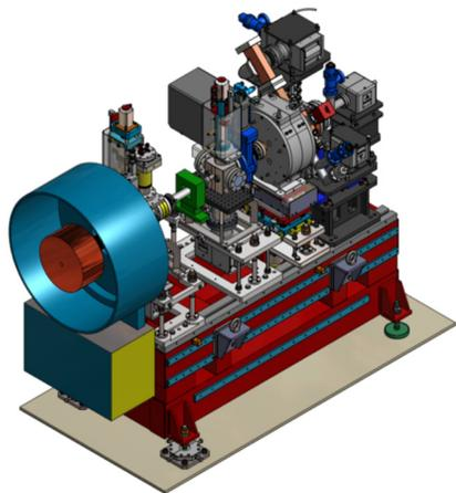
Figure 1: The new S-band RF gun schematic layout.
