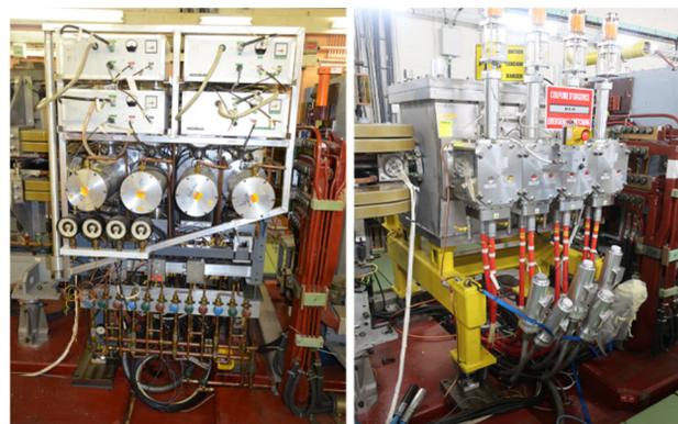
Figure 2: The old KFA45 magnet in the tunnel with s/c thyatron, TMR and oil cooling (left) and the new redesigned KFA45 in s/c configuration with the new SF6 gas free transmission cables (red) and a FC-77 filled connection box (right).
