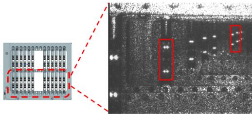
Figure 3: Glass balls mounted into the support frame and image of targets as acquired by one H-BCAM.
