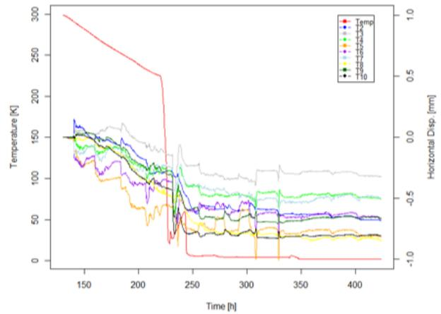
Figure 7: Targets' horizontal displacement and temperature as a function of time, B2-B4 side.
