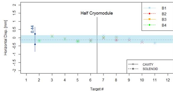
Figure 8: Targets' horizontal displacement at the end of the cooldown.
