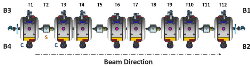
Figure 2: CAD model of prototype SSR1 string assembly. C stands for cavity, S stand for solenoid; the sequence C-S-C is repeated four times in the string assembly. The picture includes the H-BCAMs location, and targets numbering. The letter B defines the location of the four H-BCAMs.
