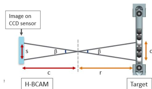
Figure 1: H-BCAMs Measurement Principle.  $d$  is a calibrated dimension ( $d = 12 \text{ mm}$ , for this design);  $s$  is the distance as measured on the charge coupled device (CCD) sensor in the H-BCAM. The ratio  $d/s$  defines the scaling factor.
