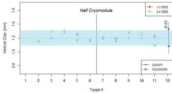
Figure 5: Targets' vertical displacement at the end of the cooldown. A positive displacement means that targets are moving down.
