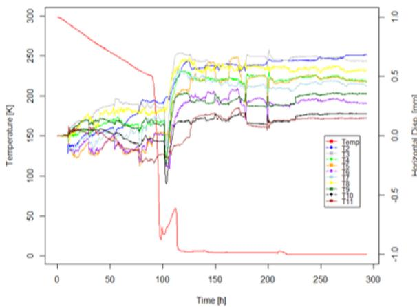
Figure 6: Targets' horizontal displacement and temperature as a function of time, B1-B3 side.
