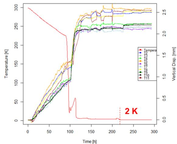
Figure 4: Targets' vertical displacement and temperature as a function of time.
