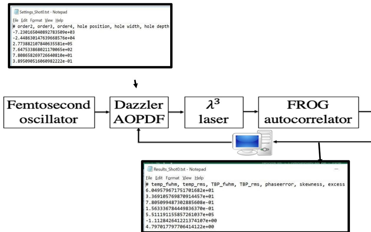
Fig. 1: A schematic of the Experimental setup. As can be seen, there are 6 input parameters which after modelling and input-output mapping predict the temporal Full width half maximum as output.
