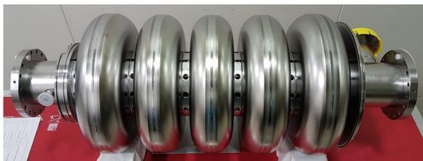
Figure 2: INFN B61\_EZ\_001 LB650 cavity for PIP-II.
