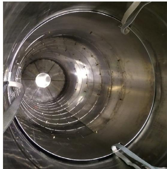
Figure 3: Cryoperm<sup>®</sup> magnetic shielding in place inside the vertical testing cryostat. A second, external shield at room temperature is placed (not visible here) around the cryostat.
