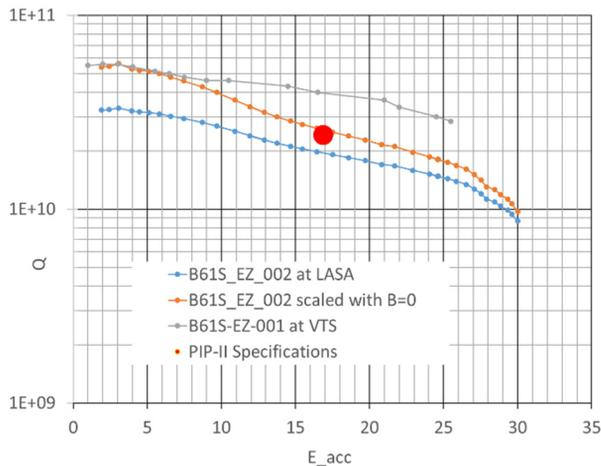
Figure 1: Q-vs- $E_{acc}$  results for the two INFN LB650 single cell cavities, compared to PIP-II specifications.
