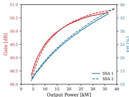
Figure 4: Sirius RF SSA towers efficiency and gain.
