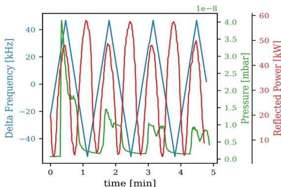
Figure 6: Cavity outgassing during RF frequency sweep conditioning.
