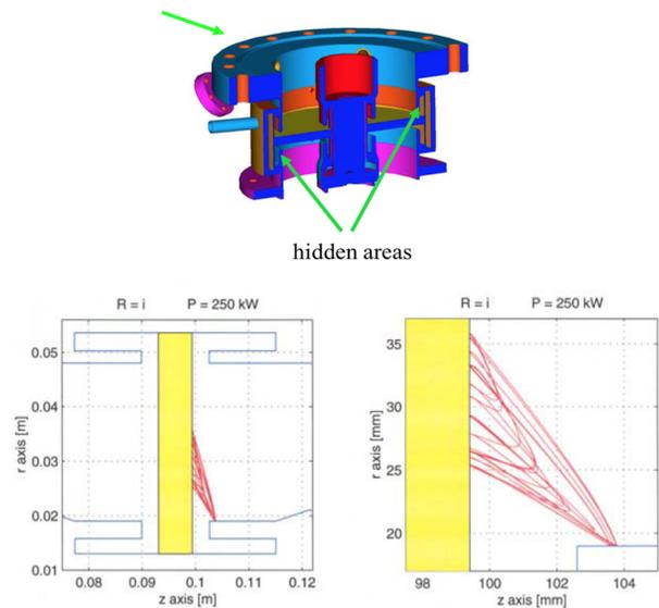
Figure 4: Coaxial choke design used at SNS [8].
