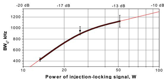
Figure 2: The admissible bandwidth of control of 2.45 GHz microwave oven magnetrons determined by measured transfer function characteristics. Black bold line shows the range and results of measurements, red lines show extrapolation with B-spline fit.
