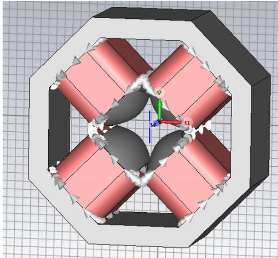
Figure 2: 3-D Model of Tapered Quadrupole Magnet.
