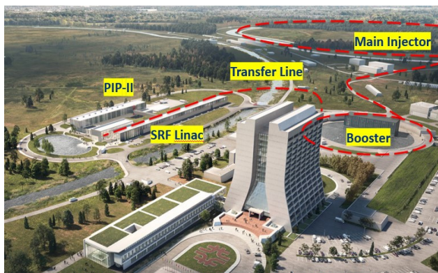
Figure 1: Fermilab PIP-II infrastructure rendering.
