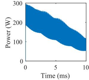
Figure 3: Time dependence of power in the first main linac cavity while ramping the injector current from 0 mA to 40 mA within 10 ms.
