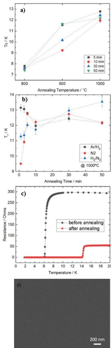
Figure 2: Effect of the post-deposition rapid thermal annealing on NbTiN film. a)  $T_c$  vs annealing temperature for different annealing times. b)  $T_c$  vs annealing time for gas atmospheres. c) Resistance vs temperature curve for NbTiN film before and after the RTA. d) SEM image of an AlN / NbTiN multilayer deposited on Si wafer by PEALD. No cracks were observed after thermal annealing.
