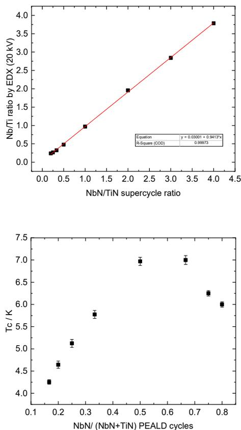
Figure 1: Linear relationship between the ratio of Nb to Ti concentration measured by EDX and the NbN to TiN ratio within the supercycle of PEALD (top) and variation of the critical temperature for the different ratios of NbN to TiN supercycles during the PEALD process (bottom).
