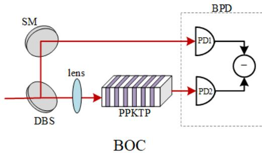
Figure 2: Main elements of BOC.
