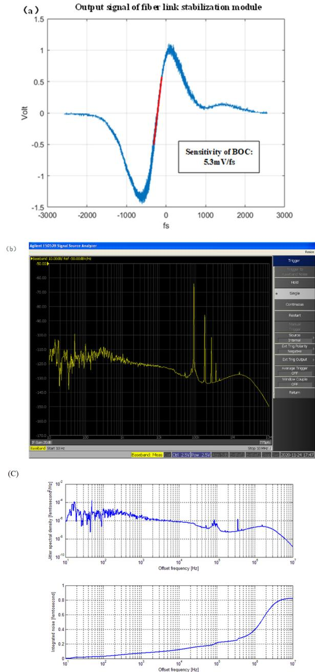
Figure 4: Experimental results of BOC: (a) output curve from the BOC and the slope shows the sensitivity about 5.3 mV/fs; (b) Noise floor result from SSA; (c) Analysis result of noise floor.
