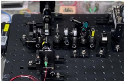
Figure 3: First version for fiber link stabilization module in lab on SXFEL.
