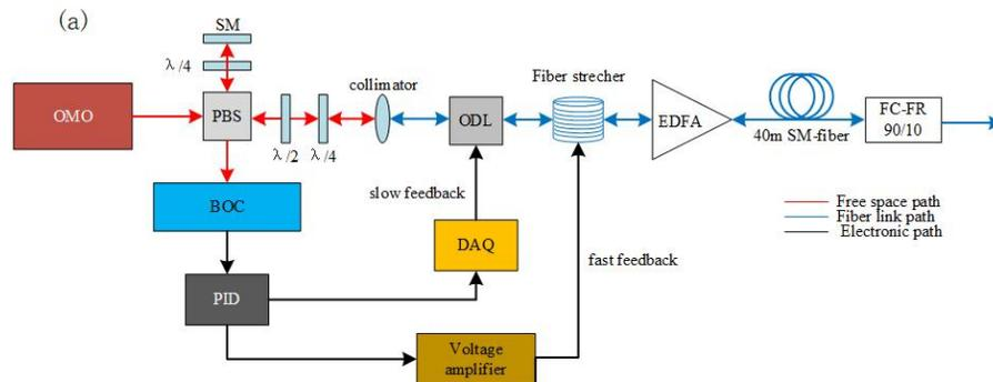
Figure 1: Schematic of the fiber link stabilization system.
