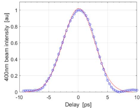
Figure 4: Measurement result for UV pulse duration.
