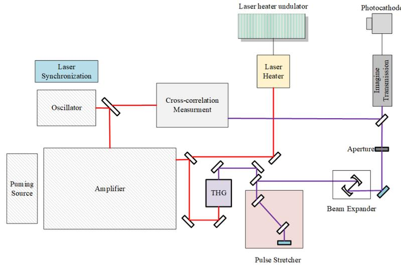
Figure 1: Schematic of SXFEL drive laser system.
