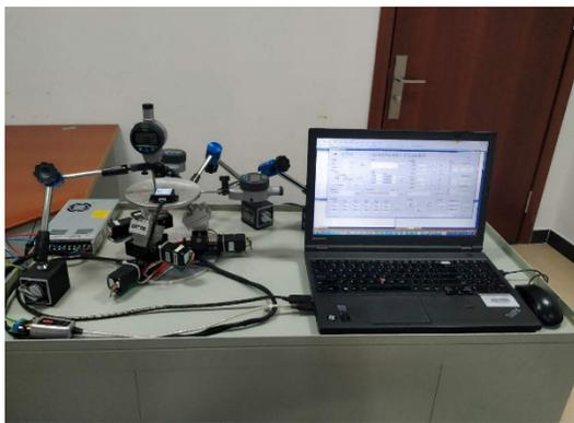
Figure 6: Positioning accuracy test of 6-DOF Platform.
