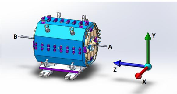
Figure 2: Schematic Diagram of Magnet Coordinate System.
